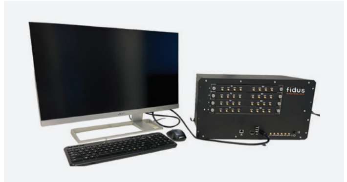
Figure 5: The Fidus RFSoc Development Platform
