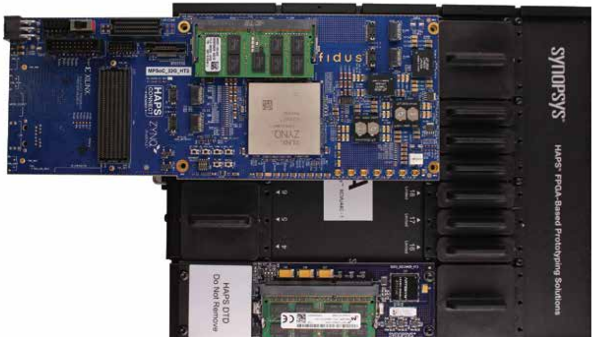
A Mantyss-32G Daughter Card mounted on a HAPS-80 Prototyping Solution
