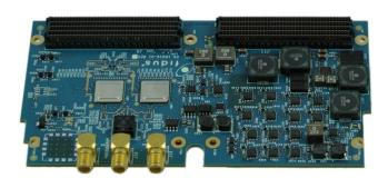
The FSF-AD15000A is a single channel analog-to-digital conversion board based on two Analog Devices AD9625 single-channel, 12-bit, 2.5 GSPS ADCs.
