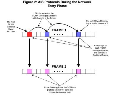
Besides the network entry phase, RATDMA and ITDMA are used in other circumstances, including interrogation responses, temporary message transmissions, request responses and binary or safety message acknowledgements. The advantage of ITDMA is that it permits the transmission of non-repeatable messages while SOTDMA can only reserve slots for repeatable messages that will continue for an extended duration (i.e. Messages 1, 2 and 9).
