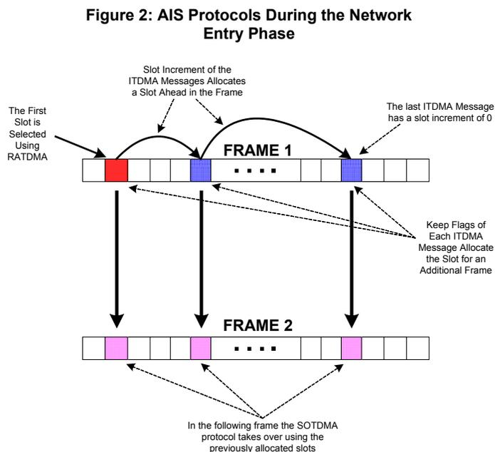
Besides the network entry phase, RATDMA and ITDMA are used in other circumstances, including interrogation responses, temporary message transmissions, request responses and binary or safety message acknowledgements. The advantage of ITDMA is that it permits the transmission of non-repeatable messages while SOTDMA can only reserve slots for repeatable messages that will continue for an extended duration (i.e. Messages 1, 2 and 9).
