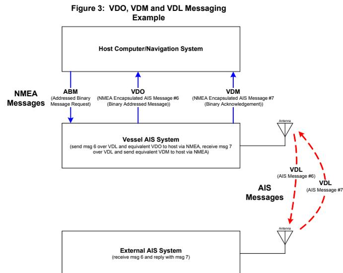
In contrast, VDM and VDO sentences are sent between a single AIS unit and the host system it is connected to. VDM and VDO sentences both consist of encapsulated AIS messages wrapped in NMEA 0183 format. Both are outputs of the AIS system. Whenever a vessel transmits an AIS message over the RF link, a corresponding NMEA 0183 sentence returns to the host. This sentence is the encapsulated "own vessel" AIS message, called VDO.
